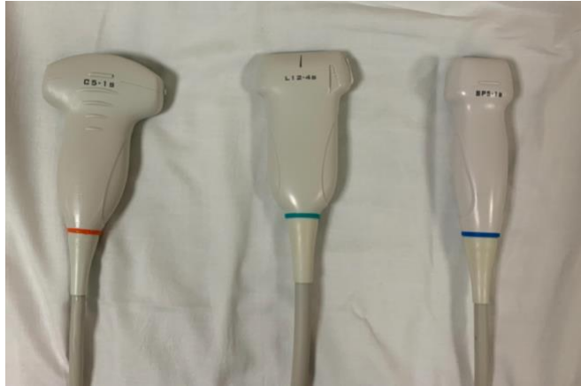
Fig. 1: Ultrasound transducers from left to right: curvilinear, linear and phased array (Image courtesy of Dr. Zachary Soucy, Dartmouth Hitchcock Medical Center)
